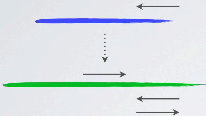
Electrons tunnel from top wire (blue) into bottom wire (green)
