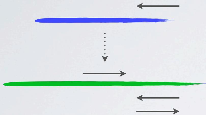
Electrons tunnel from top wire (blue) into bottom wire (green)
