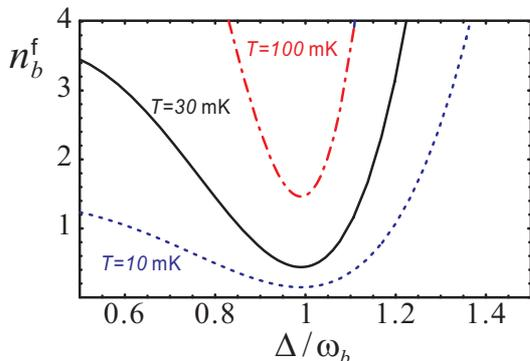
FIG. 5: (Color online) The final mean phonon number vs. effective detuning  $\Delta$  for three initial temperatures:  $T = 10 \text{ mK}$  (dotted lines),  $T = 30 \text{ mK}$  (solid lines),  $T = 100 \text{ mK}$  (dot-dashed lines). Here,  $\kappa = 0.1\omega_b$ ,  $m = 1.5 \times 10^{-13} \text{ kg}$ ,  $\omega_b = 4 \text{ MHz}$ ,  $\gamma_b = 0.25 \times 10^{-4} \omega_b$  (equivalently,  $Q_b \equiv \omega_b/\gamma_b = 4 \times 10^4$ ). For the other parameters see Fig. 2.
